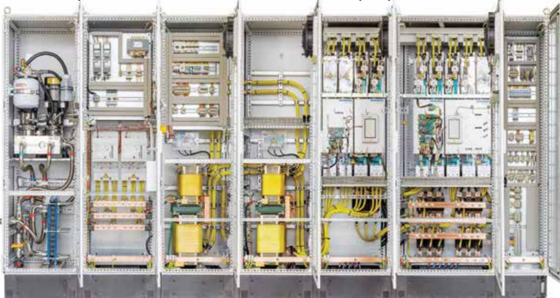
Complete 1.1MW cabinet with water-to-water cooling. Cabinet sections from left to right : 1) Cooling 2) Main switch 3) and 4) LCL filter 5) AFR with 4 PEBBs 6) VSI with 5 PEBBs 7) Aux section.
